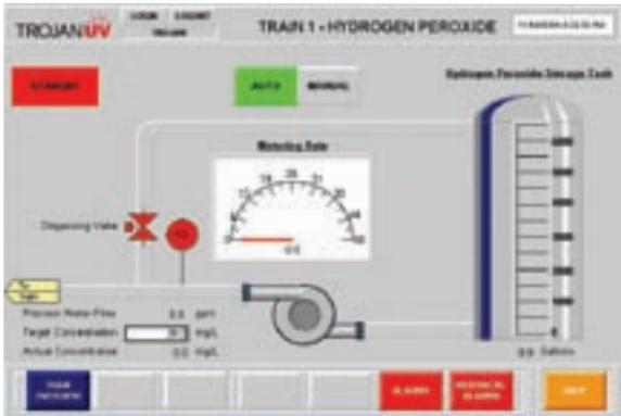
*User-friendly, integrated control systems automate delivery of UV energy and hydrogen peroxide for efficient contaminant treatment and microbial disinfection with minimal requirements of operators.*
